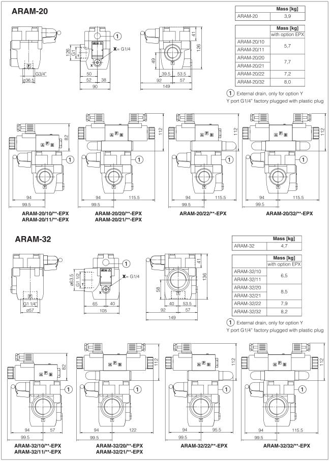
Overall dimensions refer to valves DC voltage, with connectors type 666
