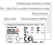
Note: **TS** values are referred to the extreme temperatures, regardless of whether the fluid or the ambient
