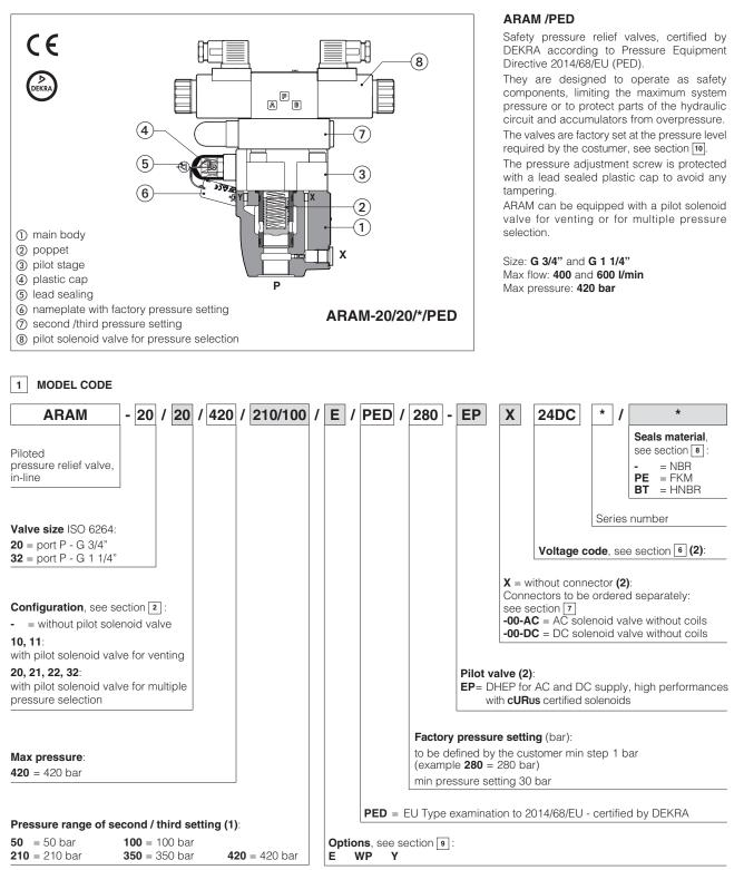
(1) Only for ARAM-\* /20, /21, /22, /32; the set pressure cannot be higher than PED factory pressure setting
