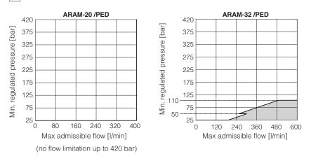
12 PERMISSIBLE RANGE - based on mineral oil ISO VG 46 at 50°C
